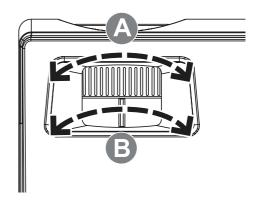
3. Use the keystone buttons to correct image distortion. They can be found on the remote control and on the projector's control panel.
