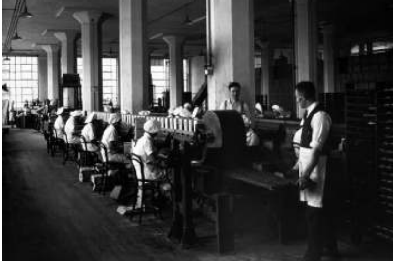
Shredded Wheat factory interior showing the packing line with a panner (on the right) feeding a pan of "Biscuits" onto the conveyor, 1926. From Where Do You Think We Worked? Image courtesy Cereal Partners UK.
